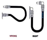
When radius is below the required minimum, use an angle adapter to avoid sharp bends.
